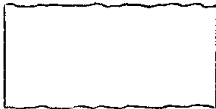
Good SSB Signal Pure Tone Input
