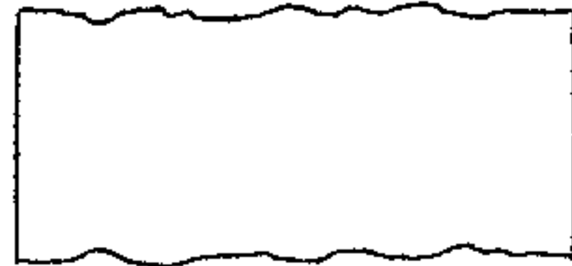
SSB Signal, Tone Input Poor Sideband Suppression
